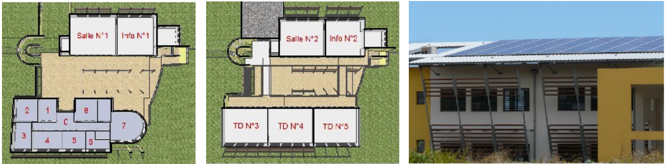
Figure 2 Ground floor (left), first floor (middle) and Northern Facade (right) of the EnerPos building. All rooms are cross-ventilated. All windows are protected by efficient wooden strips and the BIPV roof.
